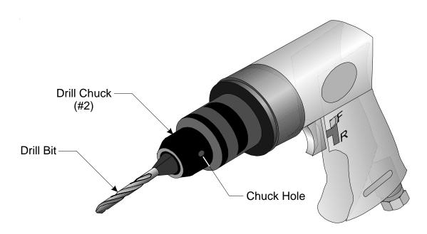
Figure 3 — Using the Chuck to Tighten the Jaws
